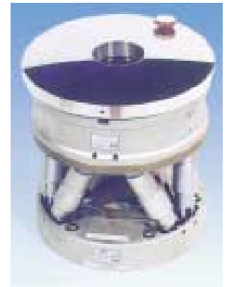
Active secondary tip/tilt mirror for the United Kingdom Infra-Red Telescope (UKIRT) on Mauna Kea, Hawaii, with Hexapod 6-degree-of-freedom alignment system (for information on Hexapod systems see the "MicroPositioners" section, p. 7-1 ff.). Mirror diameter: 314 mm Tip/Tilt range: \pm 500 \mu\text{rad} Resonant frequency: 280 Hz
