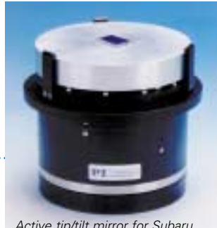
Active tip/tilt mirror for Subaru Telescope (Mauna Kea, Hawaii). Mirror diameter: 150 mm Tip/Tilt range: \pm 600 \mu\text{rad} Resonant frequency: 610 Hz
