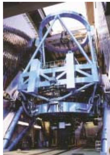
View inside the 8.2 meter optical infrared Subaru Telescope on Hawaii. From http://SubaruTelescope.org/index.html , courtesy of NAOJ.
