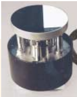
Custom tip/tilt steering mirror (100 mm diameter)
