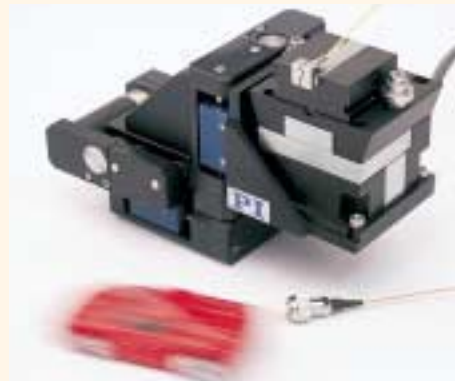
F-130 XYZ rapid-alignment system features 1 nm piezoelectric resolution and 15 mm motorized travel-range in each axis.
