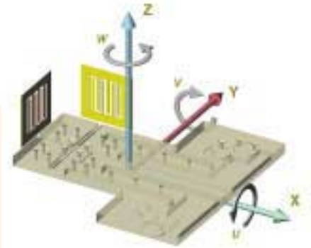
F-206 HexAlign™ Hexapod principle allows motion of platform in all six degrees of freedom. Ideal for angular scans and alignment tasks like those required in collimator packaging applications .
