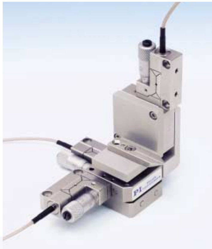
Example of an F-111-related photonics alignment system. M-313.80 XYZ stage with PiezoMike drives, 30 μm fine motion range, M-318.20 mounting bracket and F-010 V-groove fiber holder.
