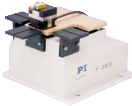
F-206 HexAlign™ 6D alignment system integrates long-travel, high-precision, six-degree-of-freedom motion and linear/rotary alignment automation. Optional high-speed, 100 \times 100 \times 100 \mu\text{m} , XYZ PZT alignment module achieves nanometer resolution.
