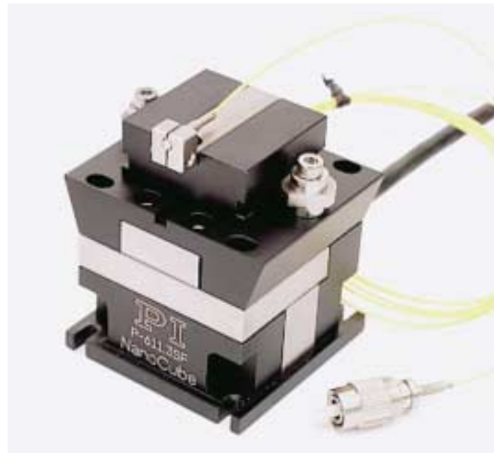
P-611 NanoCube™, XYZ Compact NanoAlignment System, 100 x 100 x 100 μm travel range, 1 nm resolution, shown with optional F-603.22 ferrule holder.
