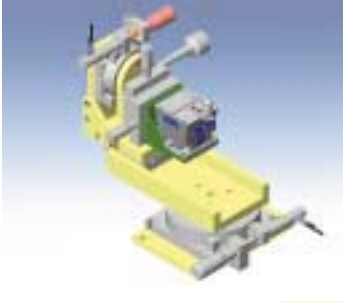
CAD design of a custom 5D coarse/fine alignment system with closed-loop PZT drives.
